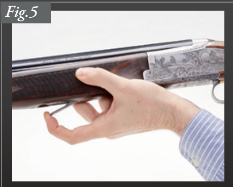
Pull outward on the forearm latch, then pivot the front of the forearm down and away from the barrels.
