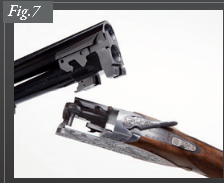
Engage the barrel lug's circular hinge pin recess with the action's hinge pin.
